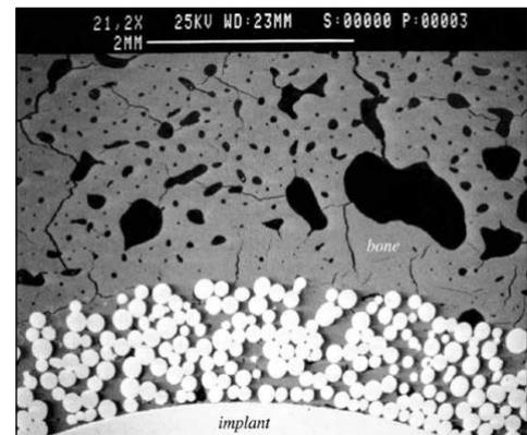
Electron microscopic photo of a porous-surfaced implant showing the bone (top gray area) growing into the beads (white) covering the implant surface.
